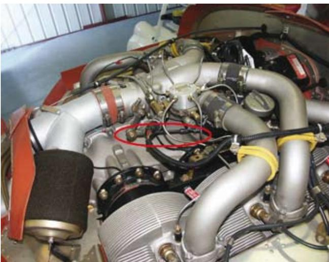
16 Exposed cables on throttle cable.
