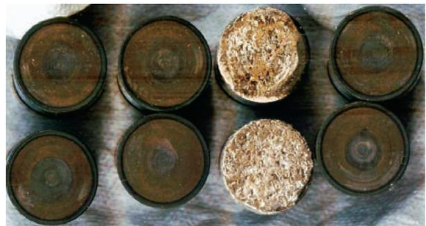
**FIGURE 2:** *If the aircraft has been inactive for months preceding the prebuy exam, it may be prudent to pull some lifters and inspect them and the cam lobes for pitting or spalling.*
