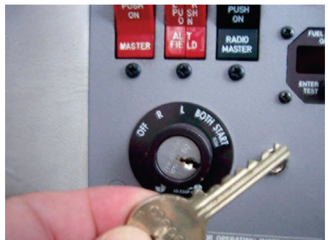
FIGURE 2: An in-flight LOP mag check is the best way to make sure your ignition system is in tip-top shape.
