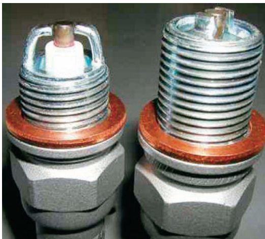
FIGURE 5: To prevent high-altitude misfire, keep plugs gapped at the tight end of the allowable range.
