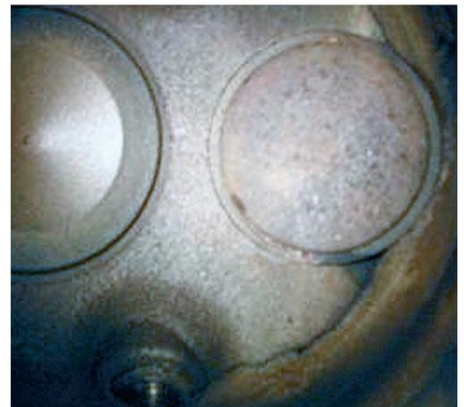
**FIGURE 2:** Cylinder head cracks are not uncommon, and become increasingly likely with increasing operating hours.
