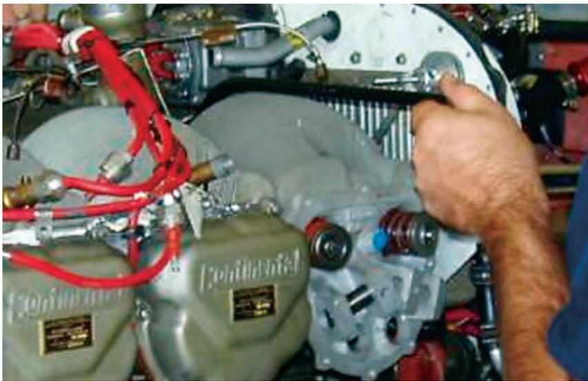
**FIGURE 3:** *Repairing or replacing a cylinder is no big deal. However, replacing all six ("top overhaul") is rarely warranted.*
