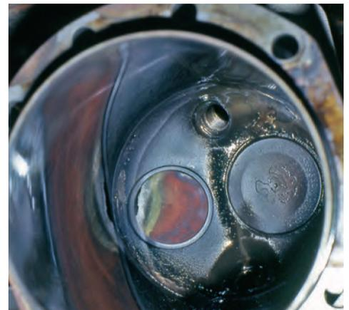
**FIGURE 1:** A "swallowed" exhaust valve, like this one, is very unlikely if you have regular borescope inspections and keep an eye on your engine monitor. But if it happens, it will definitely get your attention.
